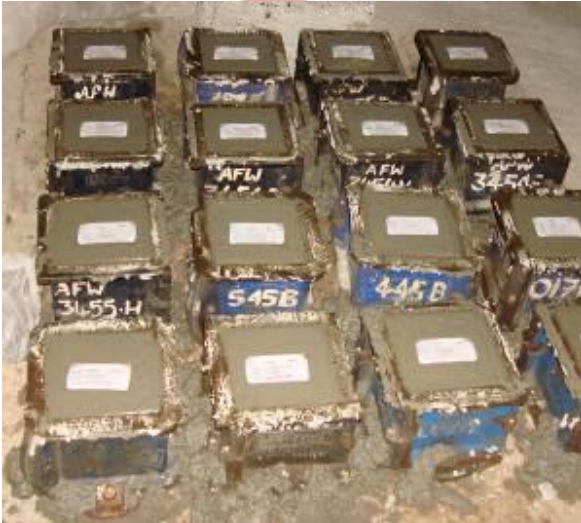
Concrete test for Wind Tower I
